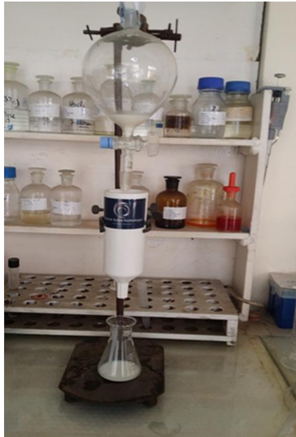
Figure 5: Preparation of treated milk after passing through device 12drops/min
